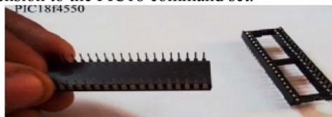
Figure 1 PIC18F4550 Microcontroller
