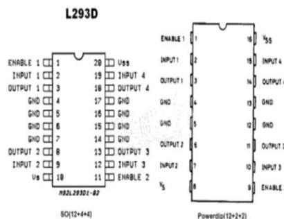
Fig. 4 Pin diagram of L293D
