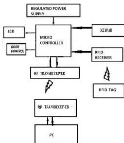
Fig 1: Architecture of Electronic Passport System
