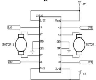
Fig. 5 DC Motor connection
