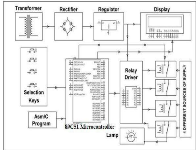
Fig.1 Block diagram of overall proposed system
