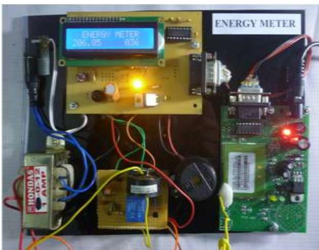
Figure 5: Hardware of energy meter
