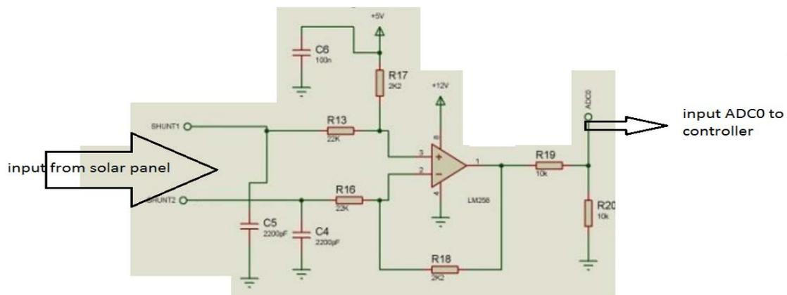
**FIG.3: Shunt resistor in series to solar panel**
