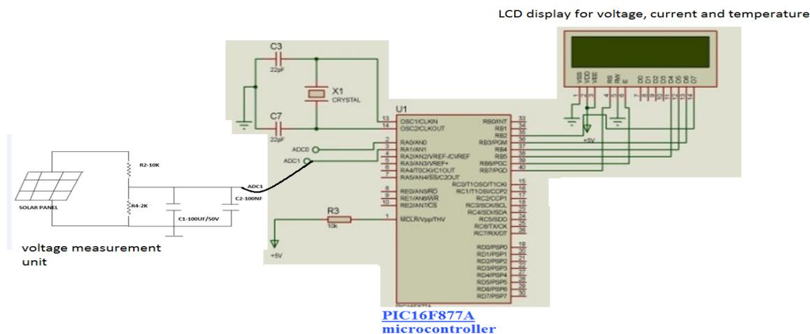
**FIG. 2: Circuit diagram for solar energy measurement system**
