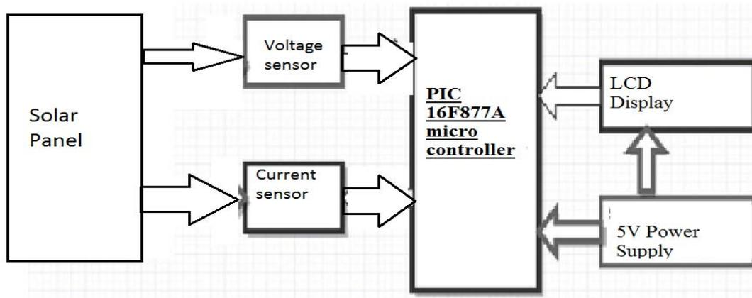
**Fig. 1. Block diagram of solar energy measurement system**
