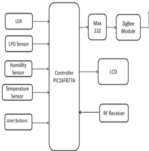
Fig. 1: Block diagram of the transmitter
