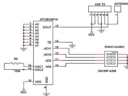
Fig. 4: Circuit diagram of the RF transmitter
