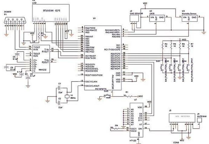
Fig. 3: Circuit diagram of the coal mine helmet as transmitter section
