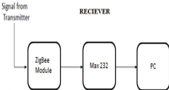
Fig. 2: Block diagram of the receiver
