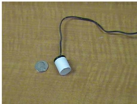
**Fig. 1: A gypsum block for moisture reading**
