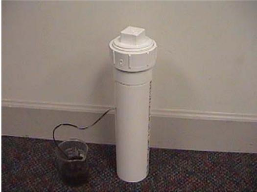
**Fig. 5: Sensor case of 3” diameter PVC**
